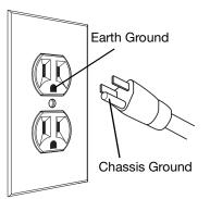
Do not use a ground-lifting adapter or cut the AC cable ground pin.
