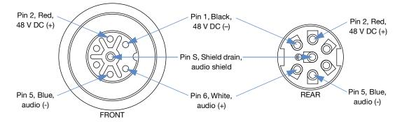
Pin Destinations for ECO-M 7-Pin Female Cable Mount Connector
