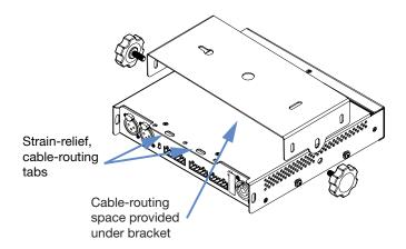
MPS-482HP Power Supply Wall Bracket Cable Routing
