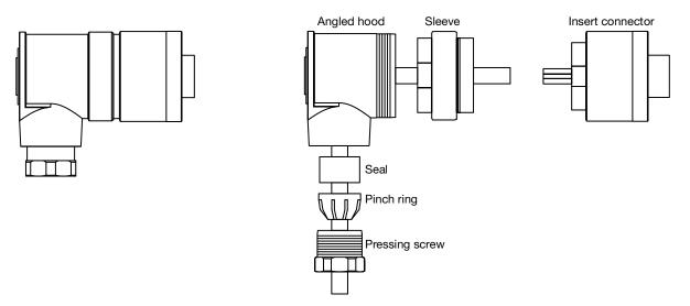
ECO-M 7-Pin Female Cable Mount Connector, Assembled (Left) and Disassembled (Right)
