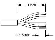
2. Insert the five exposed conductors into the five cable holes in a Phoenix 5-pin female cable mount connector. Use the following wiring scheme.
