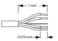
2. Insert the five exposed conductors into the five cable holes in a Phoenix 5-pin female cable mount connector. Use the following wiring scheme.
