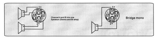
**Four-channel amplifiers** Additional connectors are provided for channel 3 and channel 4. Channel 3 functions as channel 1 above, and channel 4 as channel 2 above.
