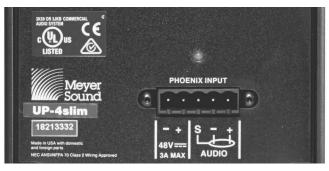
Figure 7: UP-4slim Rear Panel with Phoenix 5-pin Male Connector
