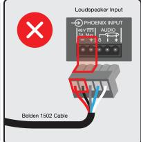
Figure 1. Incorrect, Power Supply 48 V DC Pins Connected to Audio Pins of Loudspeaker.
