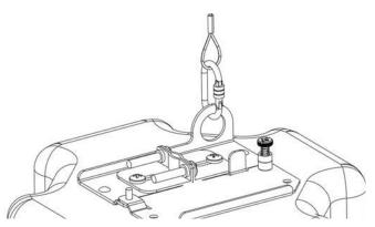
Figure 21: Attaching a safety lanyard for secondary support
