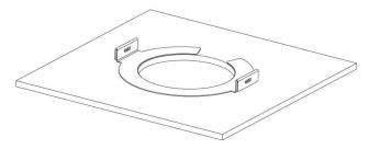
Figure 7: Using a C-ring to reinforce a brittle ceiling
