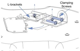
Figure 11: Removing clamping screws
