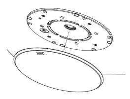
Figure 18: Placing the loudspeaker grille on the loudspeaker
