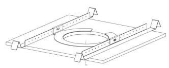
Figure 8: The C-Ring with Bridge Kit
