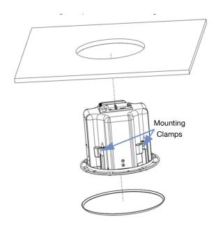
Figure 15: Inserting the loudspeaker into the ceiling
