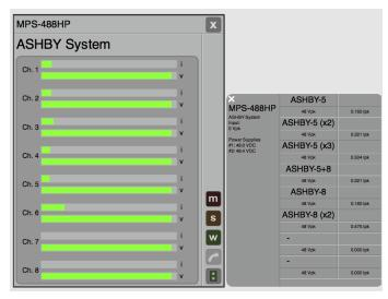
Figure 6: Voltage and current draw for connected loudspeakers in Compass
