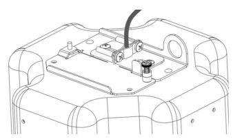
Figure 12: Clamping the wire
