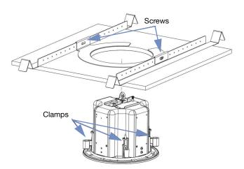
Figure 19: Installing the loudspeaker into the C-ring with Bridge Kit
