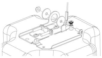
Figure 22: Attaching a safety lanyard
