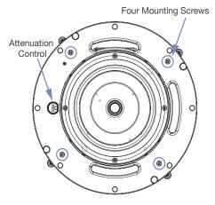
Figure 16: Ashby-5C (top) and Ashby-8C (bottom) loudspeaker mounting clamp screws and Attenuation Selector
