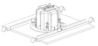
Figure 20: Installing the loudspeaker into a bridge in the ceiling
