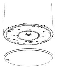
Figure 24: Fitting the grille frame onto an Ashby loudspeaker in a pendant
