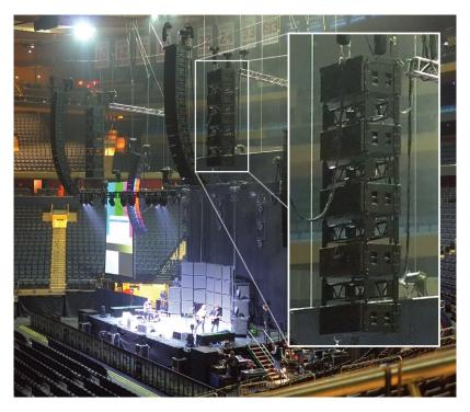
Figure 2: Cardioid Inverted Stack Gradient Array In Use—Ed Sheeran at Madison Square Garden
