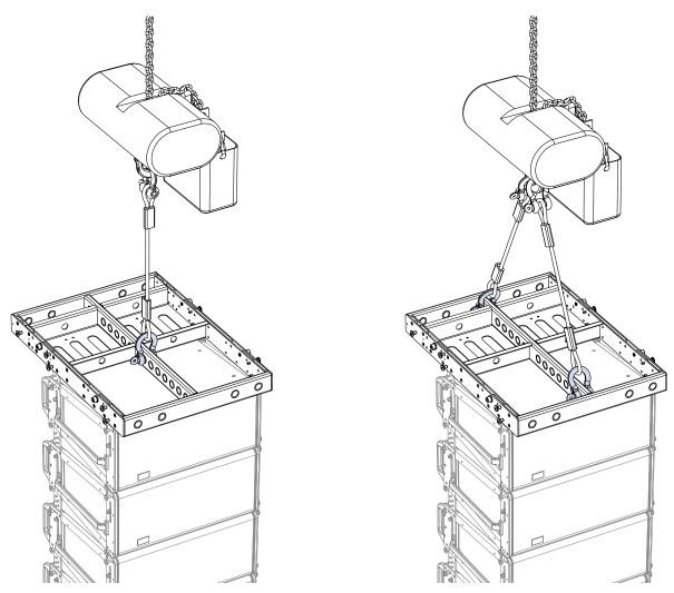
1 Motor - 1 4 Pickup Points (Left); 1 Motor - 2 Pickup Points, Front-to-Rear Bridle (Right)
