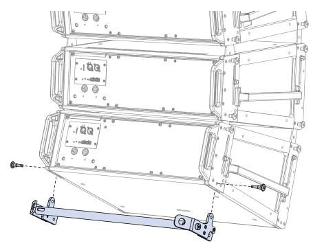
PBF-LEOPARD Pull-Back Frame Attached to Bottom LEOPARD, Exploded View
