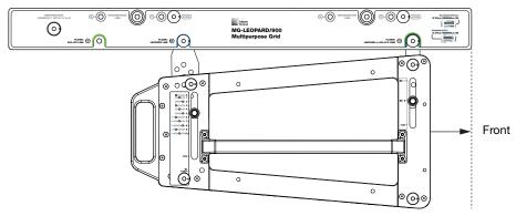
MG-LEOPARD/900-LFC Grid Oriented for Maximum Array Downtilt (Forward)
