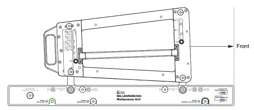
MG-LEOPARD/900-LFC Grid Oriented for Groundstack with Uptilt (Forward)
