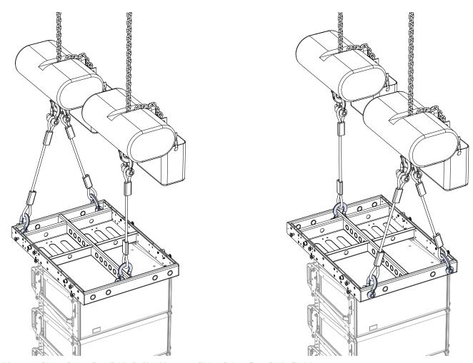
2 Motors - 3 Pickup Points, Rear Bridle (Left); 2 Motors - 3 Pickup Points, Front Bridle (Right)
