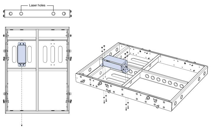
MG-LEOPARD/900-LFC Grid with Laser Bracket, Top View (Left), Exploded View (Right)
