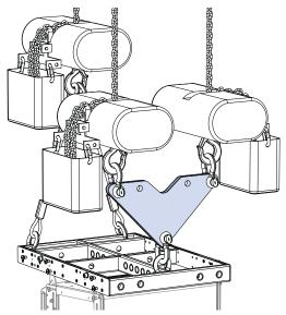
MVP Motor Vee Plate Attached to MTG-LEOPARD/900-LFC Grid
