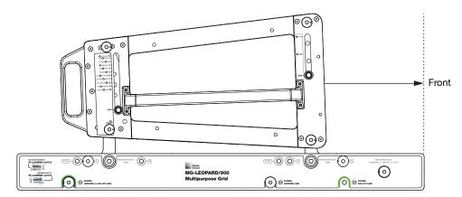
MG-LEOPARD/900-LFC Grid Oriented for Groundstack with Downtilt (Rearward)
