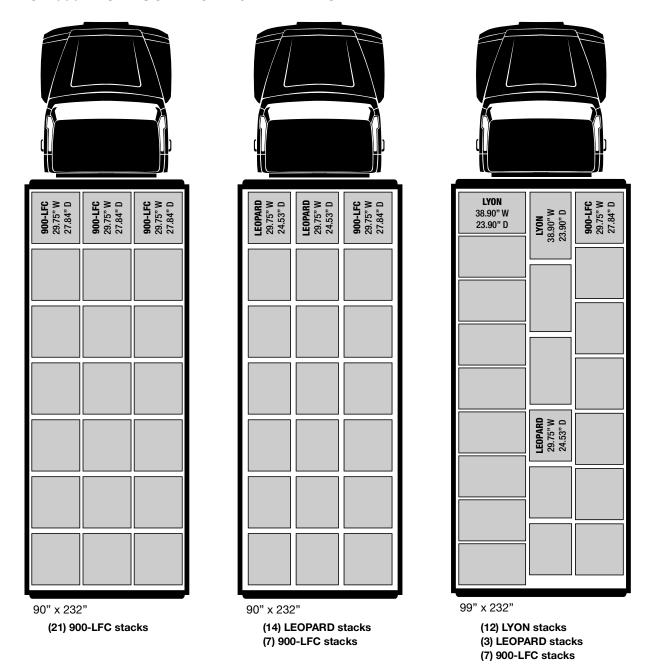
MCF-900-LFC Truck Packing Examples
