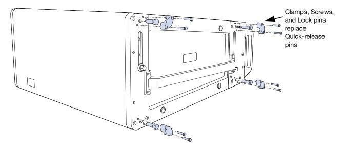
Ultra Weather Protection LEOPARD Loudspeaker Version has Clamps, Screws, and Lock pins that replace standard version quick-release pins
