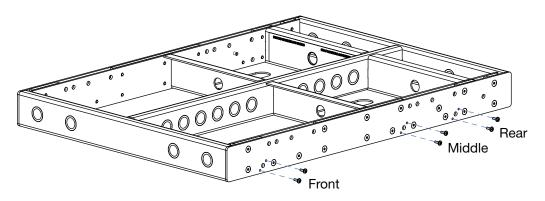
Blanking Screws (6 per side) to Prevent Corrosion at Unused Pin Locations for Ultra Weather Protection Grid
