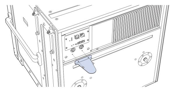
Attaching Rain Hood Baffle to LEOPARD Loudspeaker User Panel
