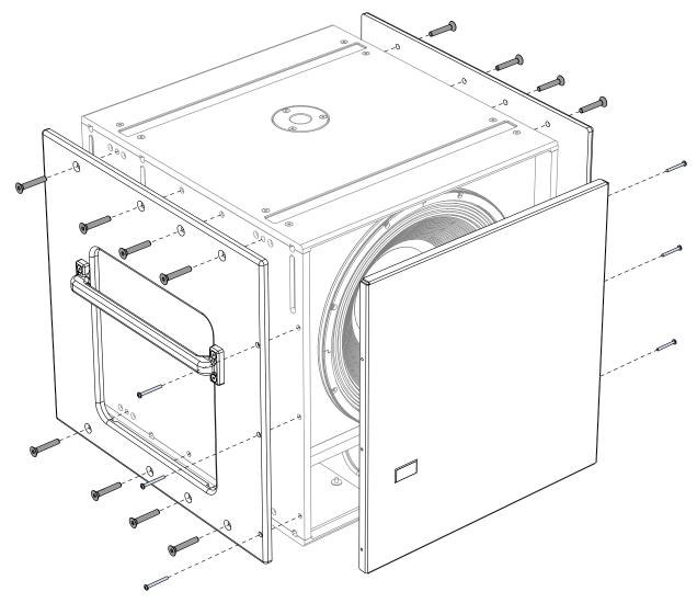
Removing Standard 900-LFC End Frames
