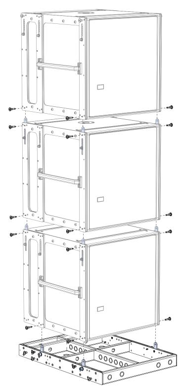
MG-LEOPARD/900-LFC Grid with Groundstacked 900-LFCs, Exploded View
