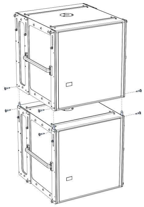
900-LFCs with MRK-900-LFC Rigging Kit, GuideALinks and Quick-Release Pins, Exploded View
