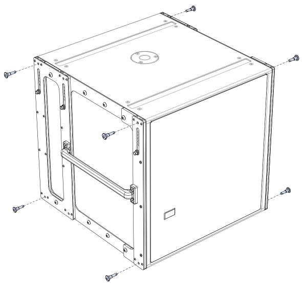
Inserting Quick-Release Pins into 900-LFC Loudspeaker Rigging
