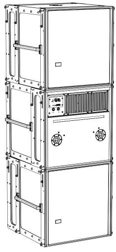
900-LFC Cardioid Groundstack (With Rigging)
