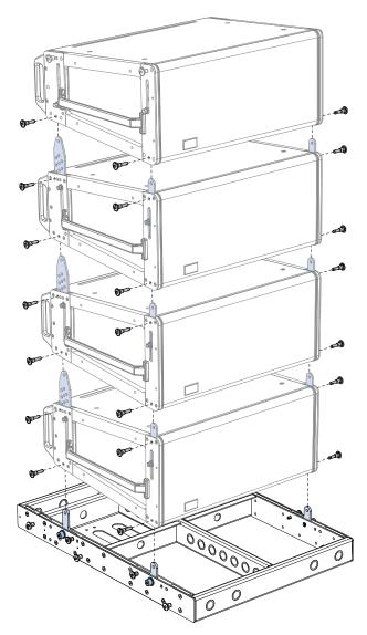
MG-LEOPARD/900-LFC Grid with Groundstacked LEOPARDs, Exploded View
