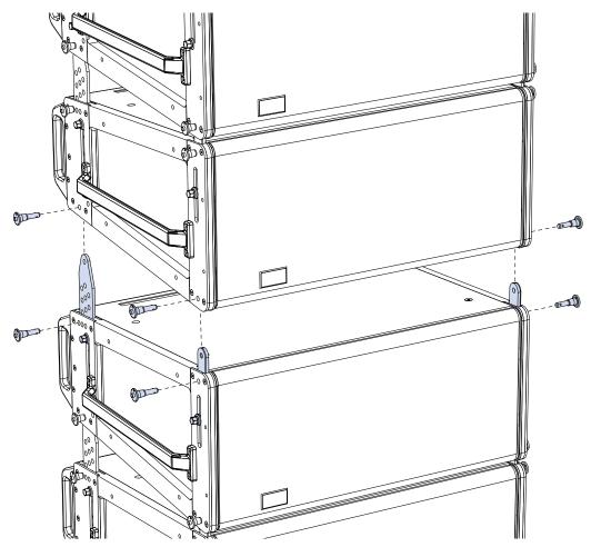
LEOPARD GuideALinks with Quick-Release Pins, Exploded View
