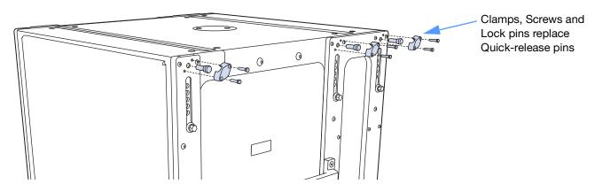
Ultra Weather Protection 900-LFC Loudspeaker Version has Clamps, Screws, and Lock pins that replace standard version quick-release pins
