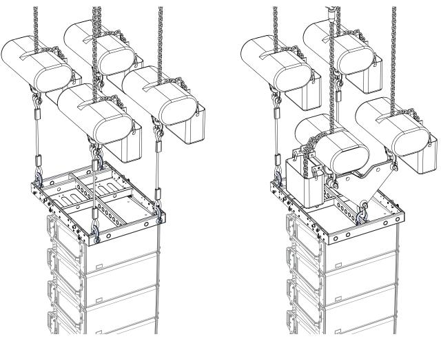
4 Motors – 4 Pickup Points (Left); 4 Motors – 3 Pickup Points, Rear Bridle, Front Vee Plate (Right)
