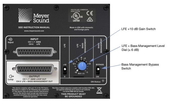
Figure 14: Physical Knob and Switches Relating to LFE and Bass Management Control
