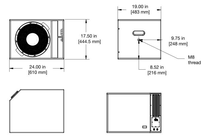
Figure 21: Amie-Sub Loudspeaker Dimensions
