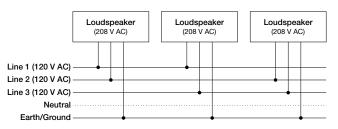
Figure 5: 120 V AC, 3-Phase Wye System (Two Lines to Loudspeakers)
