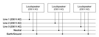
Figure 6: 230 V AC, 3-Phase Wye System (Single Line to Loudspeakers)
