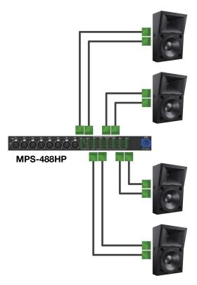
MPS-488HP with Four HMS-15 Loudspeakers
