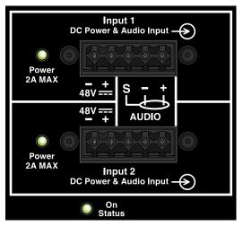
Dual-Channel Input Connectors (HMS-15)
