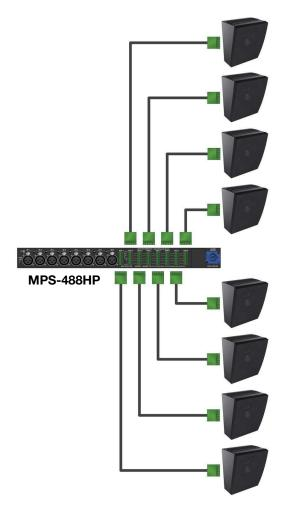
MPS-488HP with Eight HMS-10 Loudspeakers
