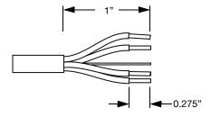
2. Insert the five exposed conductors into the five cable holes in a Phoenix 5-pin female cable mount connector. Use the following wiring scheme.
