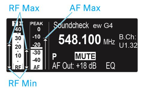
By doing a soundcheck, you can ensure adequate transmission quality in the entire area in which you want to use the transmitter. You can do the soundcheck without the help of another person.
