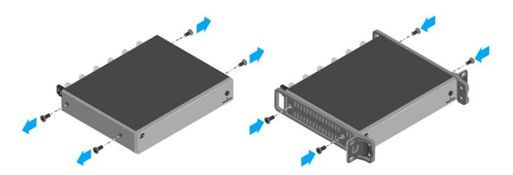
Secure the blanking plate to one of the mounting angles using two recessed head screws (M6x10).
