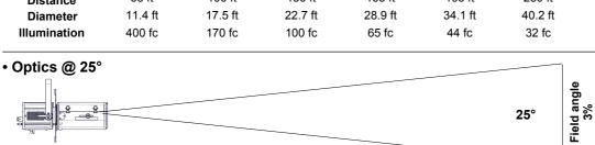
60 m 70 m **Distance** 20 m 30 m 40 m 50 m Diameter 8.9 m 13.3 m 17.7 m 22.2 m 26.6 m 31 m 130 lux Illumination 490 lux 220 lux 80 lux 55 lux 40 lux 65 ft 100 ft 130 ft 165 ft 195 ft 230 ft Distance
