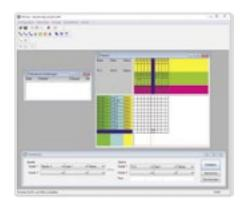
The optional VisTool touch screen software provides another method of operation. VisTool offers a visual user interface that enables additional functions such as signal metering, as well as the setting of crosspoints.
