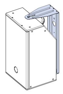
Figure 23: MUB-USW-112 Wall Mount, Vertical
