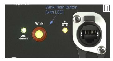
Figure 29: USW-112P Digital Audio Wink Push Button and LED
