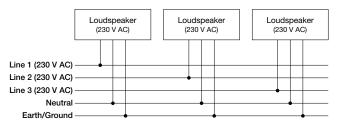
Figure 3: 230 V AC, 3-Phase Wye System (Single Line to Loudspeakers)
