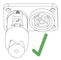
Figure 8: Locked Connector Position
