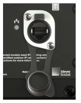
Figure 14: etherCON TOP Audio Input
