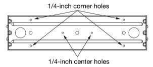
Figure 21: Mounting Hole Locations
