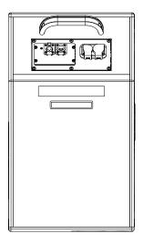
Figure 1: Only Permissible Vertical Orientation
