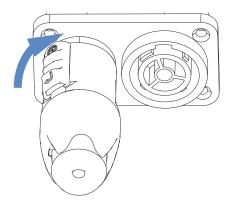
Figure 7: Rotate the Connector to Lock
