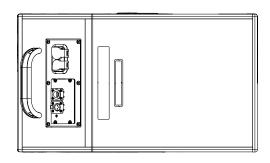
Figure 2: Only Permissible Horizontal Orientation
