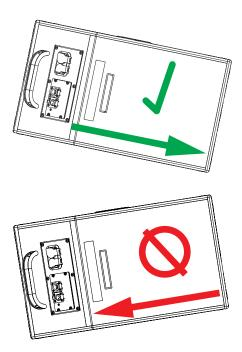
Figure 5: Horizontal Tilt-Away from Electronics Permissible (top); Horizontal Tilt-Toward Electronics **NOT** Permissible (bottom)
