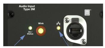
Figure 17: USW-112P On/Status LED and Ethernet connectivity LED
