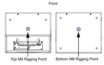
Figure 18: USW-112P Rigging Points
