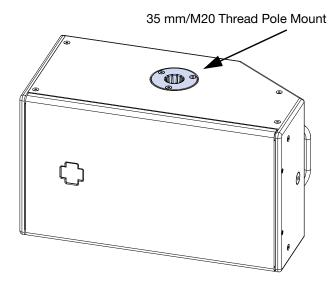
Figure 19: USW-112P Integral Pole Mount
