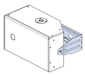
Figure 22: MUB-USW-112 Wall Mount, Horizontal
