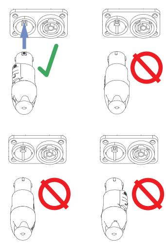
Figure 6: Proper PowerCON Connector Orientation
