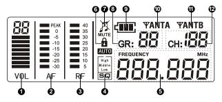
• Display meter for volume: LED bar display meter for volume and output level.
