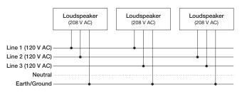
Figure 9: 120 V AC, 3-Phase Wye System (Two Lines to Loudspeakers)
