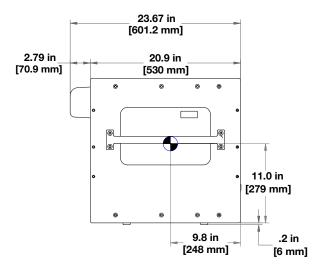
750-LFC dimensions without rigging and with rain hood installed
