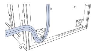
Figure 14: Cables Tied Off to Cable Ring
