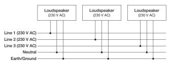
Figure 10: 230 V AC, 3-Phase Wye System (Single Line to Loudspeakers)
