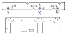
Figure 19: MG-MINA/LINA/750-LFC rigging grid
