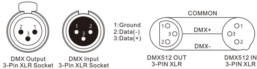
For installations where the DMX cable has to run a long distance or is in an electrically noisy environment, such as in a discotheque, it is recommended to use a DMX terminator. This helps in preventing corruption of the digital control signal by electrical noise. The DMX terminator is simply an XLR plug with a 120 Ω resistor connected between pins 2 and 3, which is then plugged into the output XLR socket of the last fixture in the chain. Please see illustrations below.
