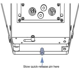
Figure 9: Stowed Quick-Release Pin, Rear Bottom
