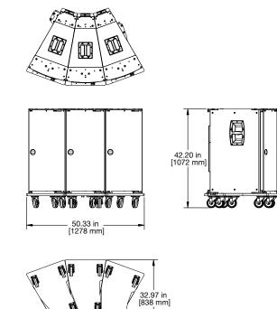
Figure 29: Dimensions for Three MDB-JM1 Dolly Boards, Normal
