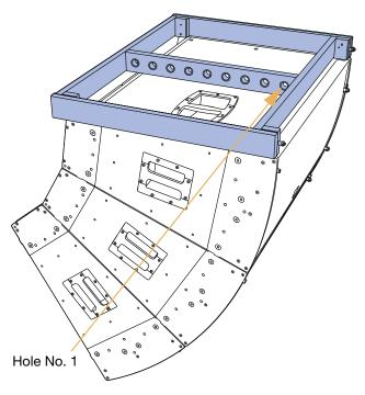
Figure 25: MTG-JM1 Vertical Grid with Three JM-1Ps
