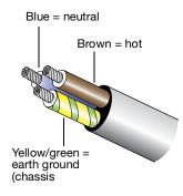
Figure 3: AC Cable Wiring Scheme
