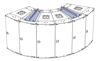
Figure 20: Two MPA-JM1 Pickup Plates with Six JM-1Ps
