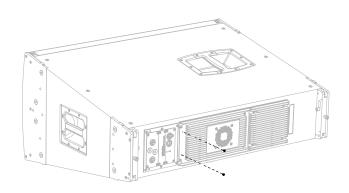
Figure 40: Removing Two Screws from Amplifier Face
