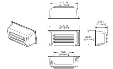
Figure 39: Horizontal Rain Hood Dimensions: Upper Rain Hood Assembly
