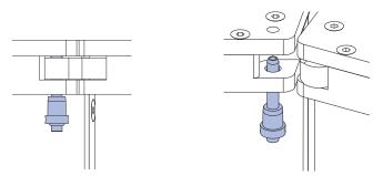
Figure 7: Rear Quick-Release Pin, GuideALink Inserted (Left); GuideALink Not Present (Right)
