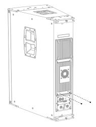
Figure 36: Removing Two Screws on Amplifier Face
