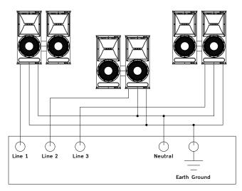
Figure 1: AC Power Distribution System
