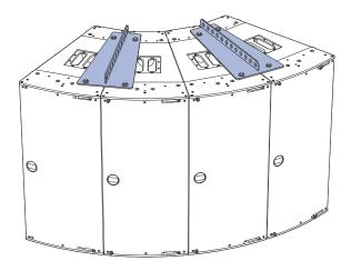
Figure 18: Two MPA-JM1 Pickup Plates with Four JM-1Ps
