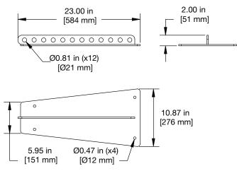
Figure 13: MPA-JM1 Pickup Plate Dimensions; Weight, 16 lbs (7.26 kg)
