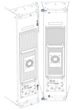
Figure 11: Inserting Rear GuideALinks
