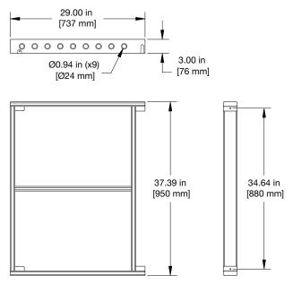
Figure 23: MTG-JM1 Vertical Grid Dimensions; Weight, 47 lbs (21.32 kg)
