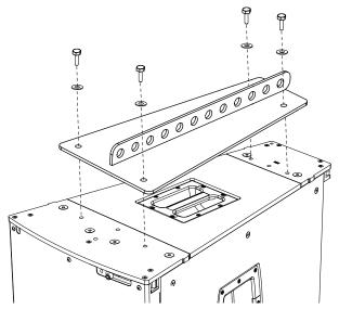
Figure 14: MPA-JM1 Pickup Plate with JM-1P
