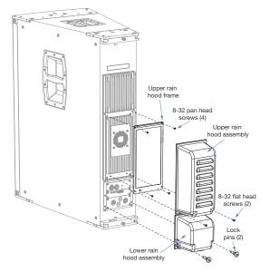
Figure 37: JM-1P Vertical Rain Hood Installation
