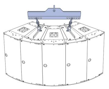
Figure 21: Two MPA-JM1 Pickup Plates with Five JM-1Ps Suspended from the MGTSB-4B Spreader Bar Using 3rd Spreader Bar Hole and 7th MPA-JM1 Pickup Plate Hole
