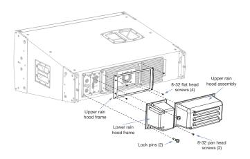
Figure 41: JM-1P Horizontal Rain Hood Installation
