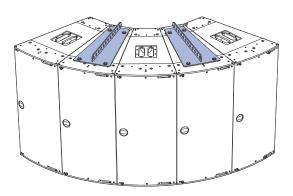
Figure 19: Two MPA-JM1 Pickup Plates with Five JM-1Ps
