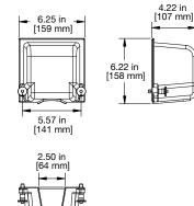
Figure 34: Vertical Rain Hood Dimensions: Lower Rain Hood Assembly
