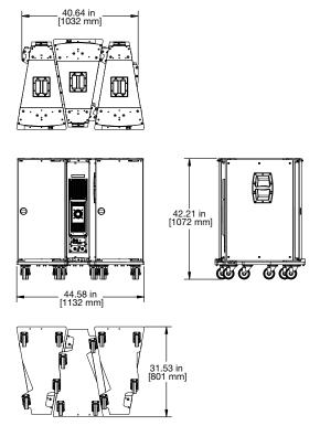
Figure 30: Dimensions for Three MDB-JM1 Dolly Boards, Staggered
