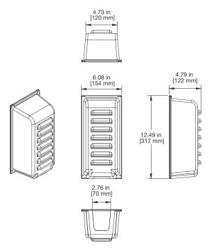
Figure 35: Vertical Rain Hood Dimensions: Upper Rain Hood Assembly (Right)
