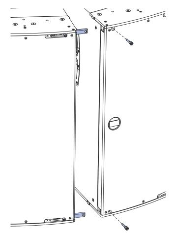
Figure 12: Inserting Front GuideAlinks
