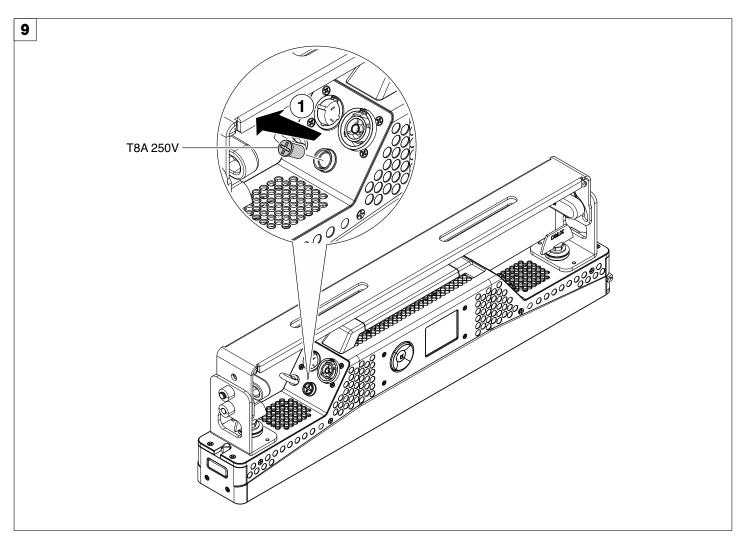
Fuse replacing - Fig. 9
