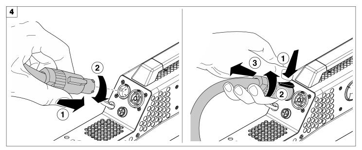
Connecting and disconnecting the power cord - Fig. 4
