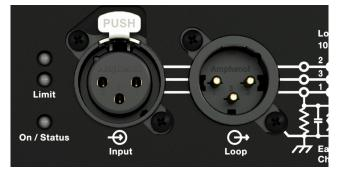
Figure 7: Audio Input and Loop Output Connectors
