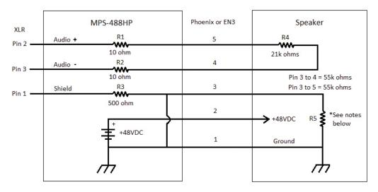
Figure 6: Power Supply to Loudspeaker Signal Flow Block Diagram
