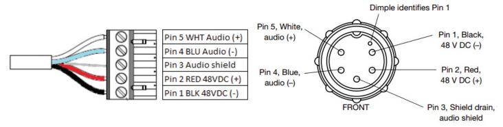
Figure 11: Phoenix Connector Pinout (left) and EN3 Connector Pinout (right)
