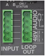
Figure 12: Ashby Loudspeaker Input Panel
