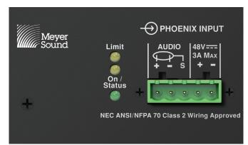
Phoenix Input Connector (Audio-Power Orientation)
