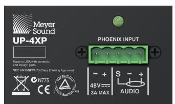
Phoenix Input Connector (Power-Audio Orientation)
