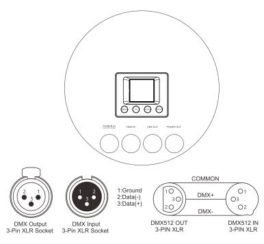
For installations where the DMX cable has to run a long distance or is in an electrically noisy environment, such as in a discotheque, it is recommended to use a DMX terminator. This helps in preventing corruption of the digital control signal by electrical noise. The DMX terminator is simply an XLR plug with a 120  $\Omega$  resistor connected between pins 2 and 3, which is then plugged into the output XLR socket of the last fixture in the chain. Please see illustrations below.
